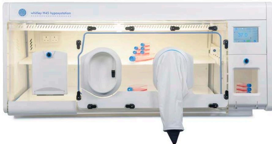
The H45 provides the facility to mimic in vivo conditions, providing a continuous cell culture environment that eliminates cellular stress linked to variations in temperature, pH levels and oxidation – resulting in better cell lines. The 3-port workstation features 2 patented oval ports, a unique Whitley Instant Access Port and has a 440 litre capacity. The 12 litre airlock will accommodate a variety of pipettes, culture flasks and electrical equipment for use in the chamber.
